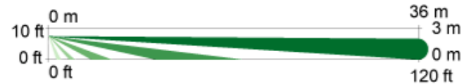
Side View Optional Long Range Coverage: 25 m to 36 m x 3 m (80 ft to 120 ft x 10 ft)
